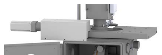
d) linear egun slide with 160mm travel in x-direction.
