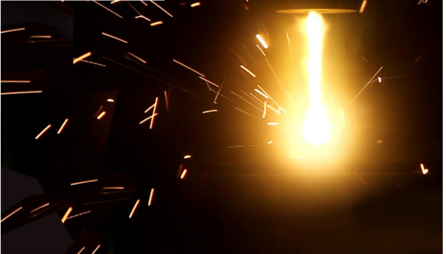
Four welds executed under 1013 mbars, 500 mbars, 100 mbars and 10 mbars: Laser beam welding with solid state lasers under low pressure shows striking results. © Foto | Institut für Füge- und Schweißtechnik der TU Braunschweig
