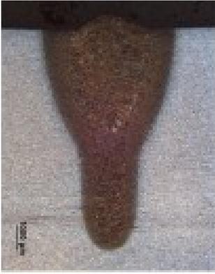
Gallery: A drop in pressure changes the shape of the seam cross section.
